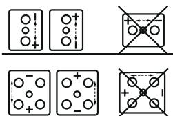
Do not invert cells (vents upside down) or allow the front of the cells to be positioned lower than the base of the cell as it might block the safety valve and damage pillars.
